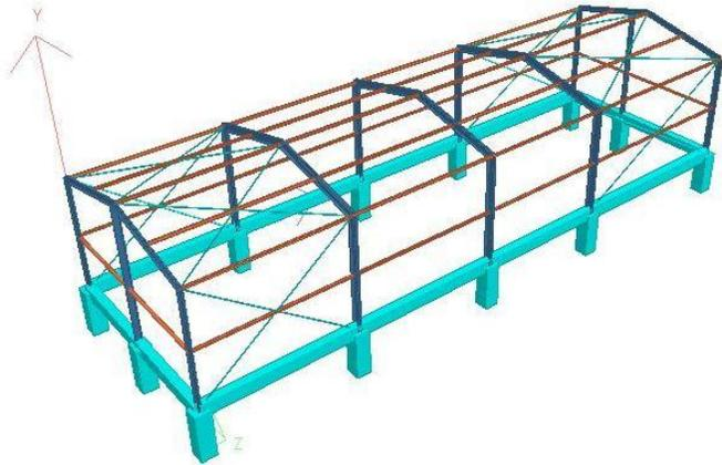
Fig 4: 3D model of a steel frame shelter
