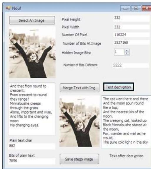
Fig. 2: The system interface showing bits statistics as well as the process of hiding sensitive text by the image based steganography.
