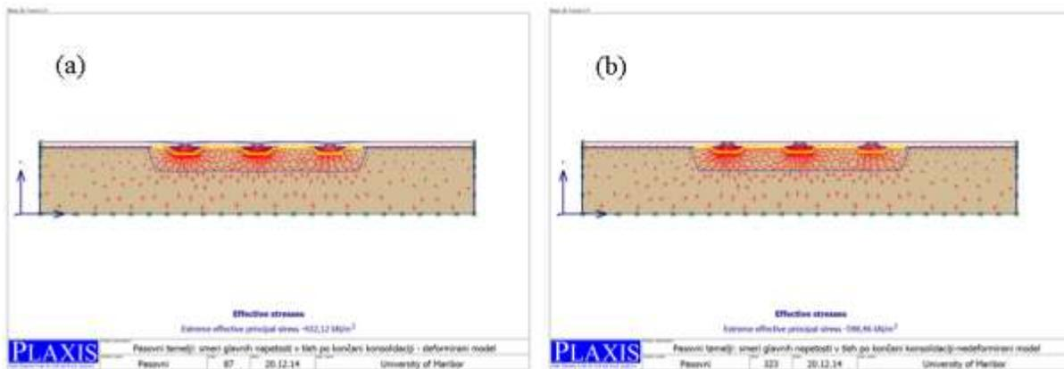
Fig 4: Trajectories of principal stresses in the soil after the end of consolidation determined by numerical analysis on the deformed elastic-plastic model  $\sigma_{max.} = 432.12 \text{ kPa}$  (a) and the undeformed elasto-plastic model  $\sigma_{max.} = 598.46 \text{ kPa}$  (b)
