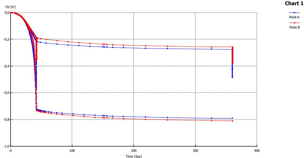
Fig 2: Vertical movement of the edge (point A) and central (point B) strip foundation as a function of time: a deformed model - the graph above, undeformed model - the graph below
