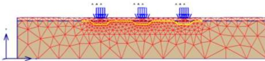
Fig 1: The system of three strip foundations
