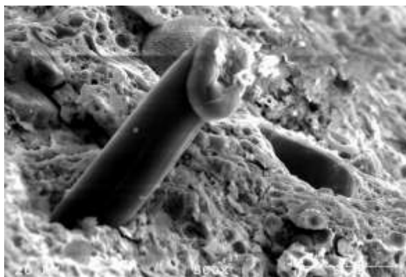
Fig. 2: SEM image obtained with the addition of 5% PP fibers at a magnification of 500 x
