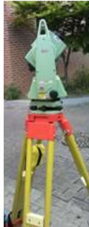
Fig. 2 : Data Acquisition System(Leica ScanStationC10)
