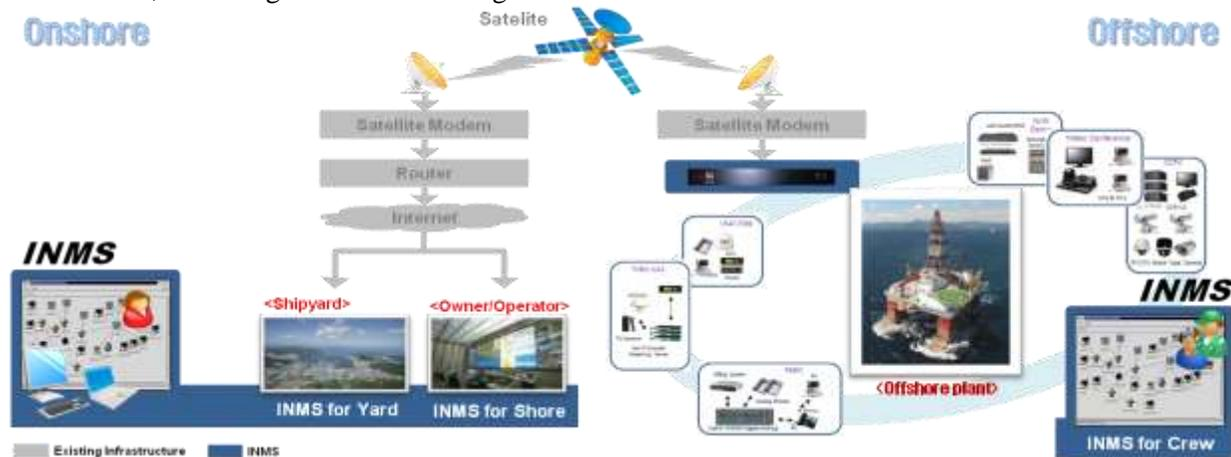
Fig. 3: Conceptual diagram of IP-based Integrated Network Management System (INMS)
