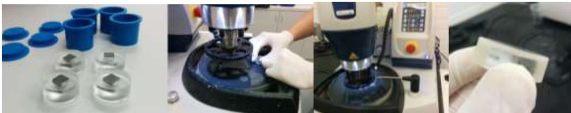
Fig. 1: Grinding and polishing of samples
