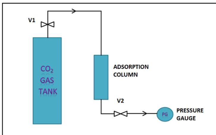
Fig. 2.1: Gas Adsorption Unit
